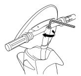
3 Tighten down the hexagonal bolt with the 6mm hexagonal wrench
